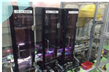
Metal chip image inspection equipment
