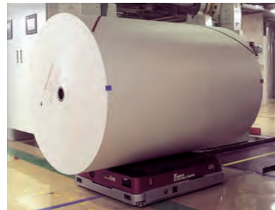
Auto Dolly Super paper roll conveying AGV
