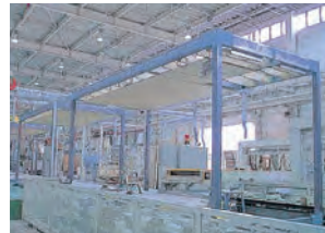
Unit conveyor Conveys components in the housing unit assembly line.
