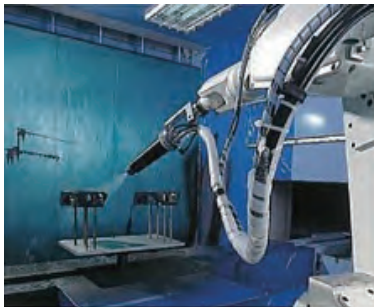
Painting robot, internal pressure automatic control booth
