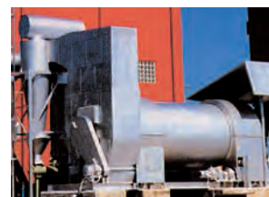
Sludge drying system
