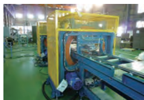
Shrink wrapper Can wrap items on four or six sides.
