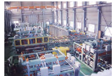
Exterior wall board packing line Integrated line for accumulation, stacking, packing, palletizing, and other processes.
