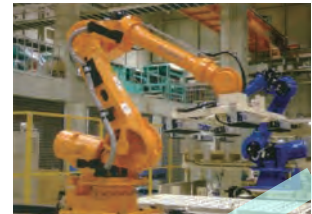
Robotic handling A robot with traveling axes depalletizes and conveys boards, and another robot affixes boards to the housing units.
