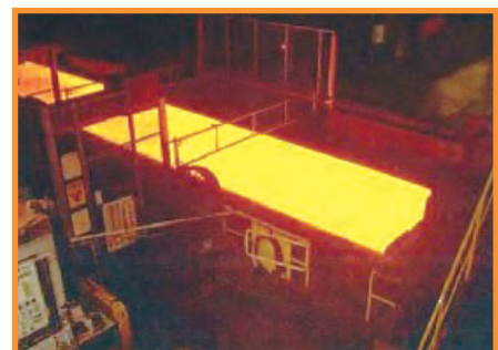
Post-rolling cooling conveyor
