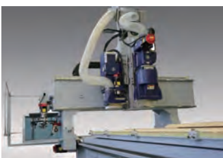
Exterior-wall cutting machine Cuts exterior walls, rebar included. Comes with dust collector.
