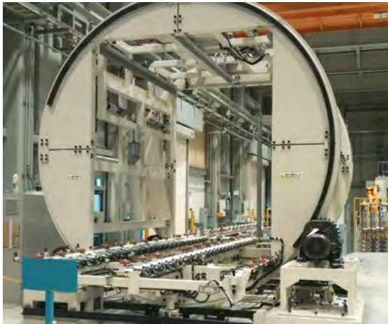
Unit turnover machine Turns over frames and panels.
